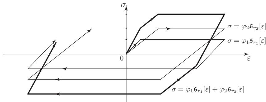
Figure 2: The stop operators and their combinations.
