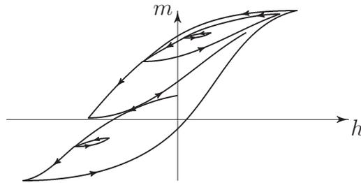
Figure 1: Hysteresis in ferromagnetism.
