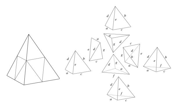
Figure 3: Red refinement of a tetrahedron T by plane cuts through midlines of its faces (left) and its exploded version (right).
